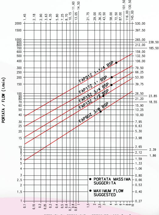
PERDITA DI PRESSIONE / PRESSURE LOSS (bar)
