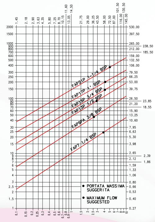
PERDITA DI PRESSIONE / PRESSURE LOSS (bar)
