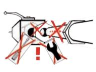
**Don't operate a ball valve with a tool or an extension**
