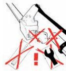
**Don't operate a ball valve with a tool or an extension**
