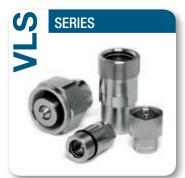
Valving style: **Poppet** Interchange: **Similar Couplings** Available sizes: **From 1/2" to 1"** Operating pressure: **Up to 465 bar** Flow rate: **Up to 200 L/Min** Material: **High strength carbon steel** Connection system: **Screw** Connection under pressure: **One side** Typical use: **Outdoor**
