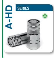
Valving style: Flat face Interchange: ISO 16028 -NFPA T3.20.15 - HTMA (size 3/8") Available sizes: From 3/8" to 1/2" Operating pressure: Up to 350 bar Flow rate: Up to 90 L/Min Material: High strength carbon steel Connection system: Push Connection under pressure: Female side, other side to drain Typical use: Outdoor
