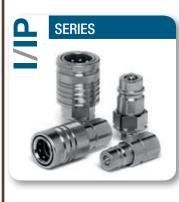
Valving style: Poppet (Breakaway system) Interchange: ISO 7241-1 A Available sizes: From 1/4" to 1" Configuration: Modular construction Operating pressure: Up to 350 bar Flow rate: Up to 200 L/Min Material: High strength carbon steel Connection system: Push-pull Connection under pressure: Not allowed Typical use: Outdoor
