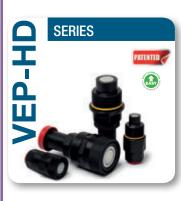
Valving style: Flat face Interchange: Stucchi profile Available sizes: From 3/4" to 1-1/2" Operating pressure: Up to 500 bar Flow rate: Up to 750 L/Min Material: High strength carbon steel Connection system: Screw Connection under pressure: Both side, easy connection + disconnection allowed Typical use: Outdoor (Heavy duty)
