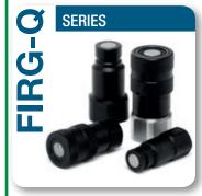
Valving style: Flat face Interchange: ISO 16028 -NFPA T3.20.15 - HTMA (size 3/8") Available sizes: From 1/4" to 2" Operating pressure: Up to 300 bar Flow rate: Up to 1000 L/Min
