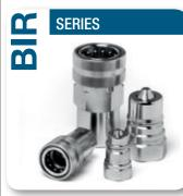
Valving style: **Poppet** Interchange: **ISO 7241-1 A** Available sizes: **From 1/4" to 2"** Operating pressure: **Up to 350 bar** Flow rate: **Up to 1000 L/Min** Material: **High strength carbon steel** Connection system: **Single acting sleeve** Connection under pressure: **One side with PC version** Typical use: **Outdoor**
