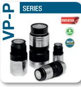
Valving style: Flat face Interchange: Stucchi profile Available sizes: From 1/4" to 1-1/2" Operating pressure: Up to 600 bar Flow rate: Up to 750 L/Min Material: High strength carbon steel Connection system: Screw Connection under pressure: Both side, easy connection + disconnection allowed
