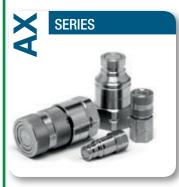
Valving style: Flat face Interchange: ISO 16028 -NFPA T3.20.15 - HTMA (size 3/8") Available sizes: From 1/4" to 1" Configuration: Modular construction Operating pressure: Up to 350 bar Flow rate: Up to 378 L/Min Material: Stainless steel (AISI 316) Connection system: Push Connection under pressure: Not allowed Typical use: Indoor & Outdoor
