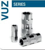
Valving style: Check valves Available sizes: From 1/8" to 2" Standard cracking pressure: Up to 4,5 bar Flow rate: Up to 1000 L/Min Material: High strength carbon steel Typical use: Outdoor
