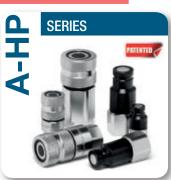
Valving style: Flat face Interchange: Stucchi profile Available sizes: From 1/8" to 3/8" Operating pressure: Up to 720 bar Flow rate: Up to 46 L/Min Material: High strength carbon steel Connection system: Push Connection under pressure: Not allowed Typical use: Outdoor
