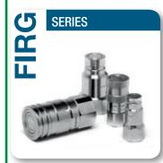
Valving style: Flat face Interchange: ISO 16028 -NFPA T3.20.15 - HTMA (size 3/8") Available sizes: From 1/4" to 2" Operating pressure: Up to 300 bar Flow rate: Up to 1000 L/Min Material: High strength carbon steel Connection system: Push Connection under pressure: Not allowed Typical use: Outdoor
