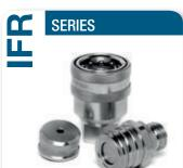
Valving style: Flat face Interchange: ISO 5676 Available sizes: 3/8" Operating pressure: Up to 150 bar Flow rate: Up to 23 L/Min Material: High strength carbon steel Connection system: Single acting sleeve Connection under pressure: Not allowed Typical use: Outdoor
