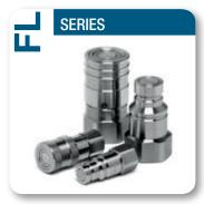
Valving style: Flat face Interchange: ISO 16028 -NFPA T3.20.15 - HTMA (size 3/8") Available sizes: From 1/8" to 2" Operating pressure: Up to 350 bar Flow rate: Up to 1000 L/Min Material: Stainless steel (AISI 316) Connection system: Push Connection under pressure: Not allowed Typical use: Indoor & Outdoor
