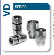
Valving style: **Poppet** Interchange: **ISO14541** Available sizes: **From 1/4" to 1-1/4"** Operating pressure: **Up to 450 bar** Flow rate: **Up to 378 L/Min** Material: **High strength carbon steel** Connection system: **Screw** Connection under pressure: **One side** Typical use: **Outdoor**
