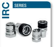
Valving style: **Poppet** Interchange:**similar couplings** (Nordic interface) Available sizes: **From 1/4" to 1"** Operating pressure: **Up to 600 bar** Flow rate: **Up to 378 L/Min** Material: **High strength carbon steel** Connection system: **Single acting sleeve** Connection under pressure:
