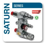
Valving style: Flat face Interchange: ISO 16028 (for the couplings) Available sizes: From 1/2" to 3/4" Operating pressure: Up to 350 bar Flow rate: Up to 200 L/Min Material: High strength carbon steel Connection system: Push Connection under pressure: One side+disconnection allowed Typical use: Outdoor
