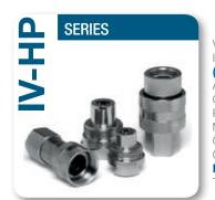
Valving style: **Ball** Interchange: **Similar Couplings (High Pressure)** Available sizes: **From 1/4" to 3/8"** Operating pressure: **Up to 700 bar** Flow rate: **Up to 23 L/Min** Material: **High strength carbon steel** Connection system: **Screw** Connection under pressure: **Not allowed** Typical use: **Outdoor**
