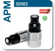
Valving style: Flat face Interchange: ISO 16028 -NFPA T3.20.15 - HTMA (size 3/8") Available sizes: From 3/8" to 1-1/2" Operating pressure: Up to 350 bar Flow rate: Up to 750 L/Min Material: High strength carbon steel Connection system: Push Connection under pressure: Male side, other side to drain Typical use: Outdoor
